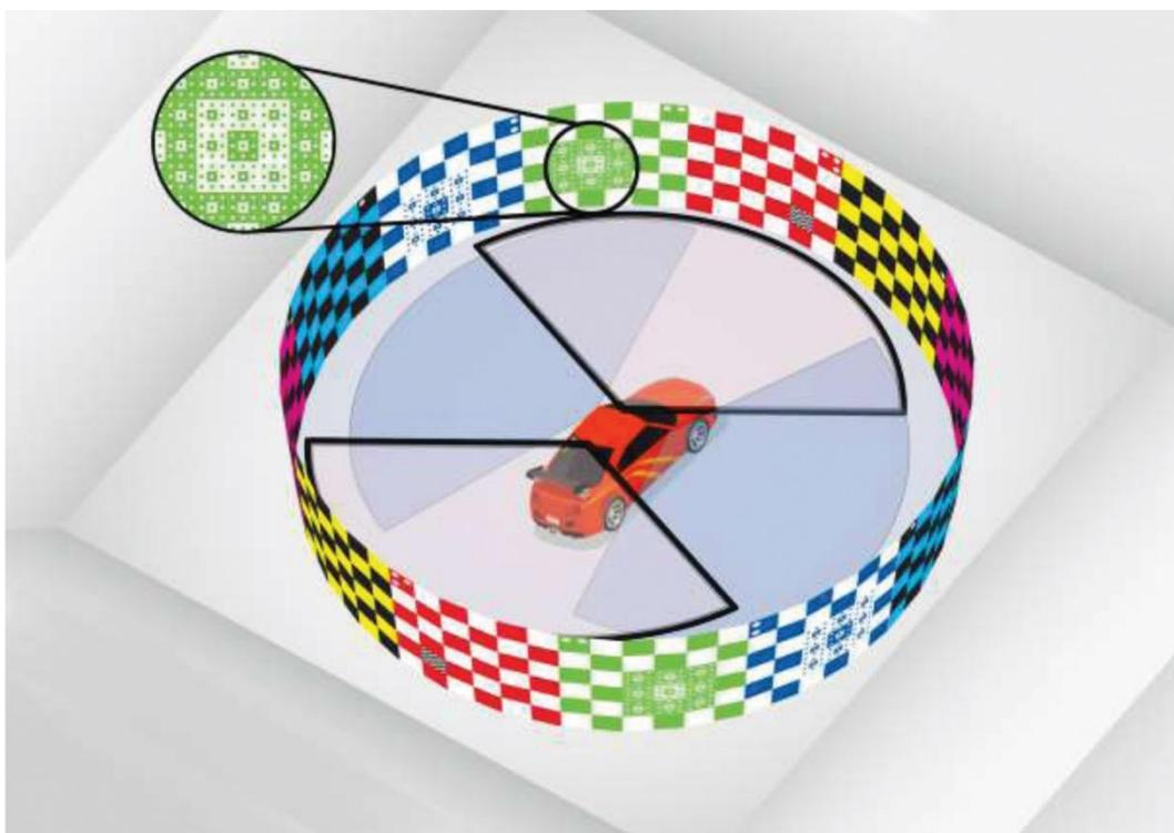
**Fig 1:** The calibration tunnel covered by 360° pattern. The fractal shape is magnified.
